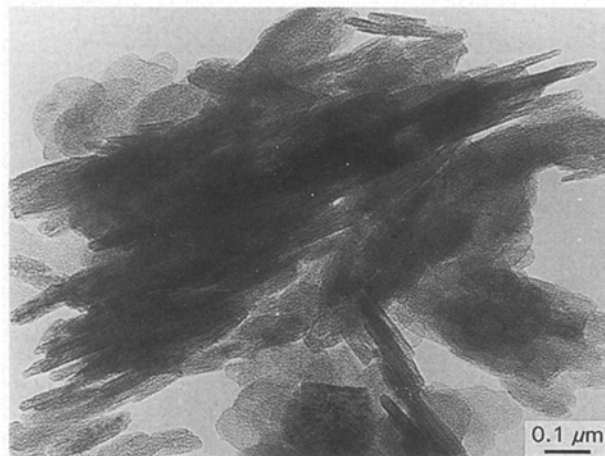
Figure 6 Transmission electron micrograph of magnesium hydroxide particles.
